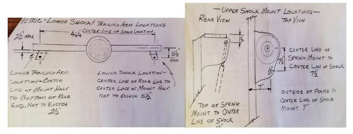
Full Size chassis 112" & 116": 3.25 inches from center trailing arm to center shock.
